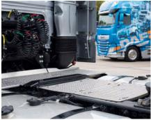
full air suspension, as does the next step up, the Low, which has an 850mm frame height. Wider 355/50 tyres are also an option for the front axle.
